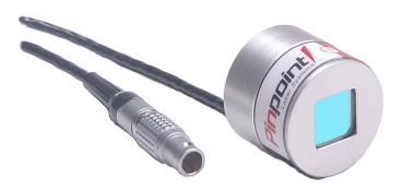
The Microgage Disc Receiver is compact and will fit into small places for bore alignment, checking extruder barrels, shaft bearings and much more. The method of operation is simple a narrow laser beam provides a measuring reference line and this receiver will determine
