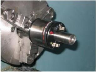
held in the chuck. The laser beam then travels some distance down the length of the machine before it reaches the Microgage Receiver. If the chuck does not grip the laser shank evenly or if there is any reason that the laser doesn't sit squarely in it's mounting
