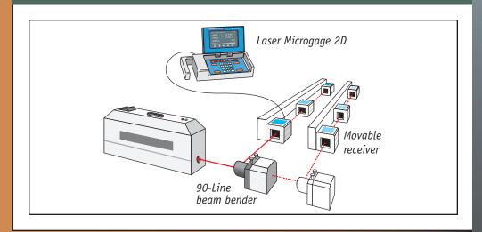
Easily achieve pairs of parallel lines by moving the 90-Line Right Angle to different locations along the beam path and comparing readings along each line. Check assemblies, align rolls and idlers, adjust web systems, position tracks and guide rails, adjust gantry and stage systems, position moving slides, and other applications.
