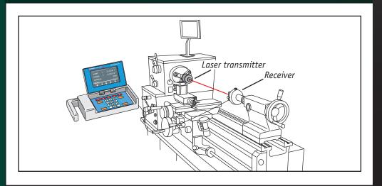
Placing a laser in a machine tool spindle or collet or in a lathe chuck projects a precise laser reference line for measurements. Locating the Microgage receiver on the tool holder, tailstock, bar feeder, and other machinery elements is a precise and easy way to check alignment and verify that the machine runs straight and true. These quick, precise measurements are ideal for lathes, CNC turning centers, boring machines and other spindle based tools.
