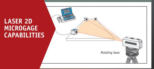
Set the laser transmitter on our adjustable rotating base to define a flat plane of laser light for measuring surface flatness and aligning components and assemblies in a precise plane. Perfect for profiling machine beds, adjusting web and roller systems, checking gantry travel, setting tracks and rails, and positioning machinery.
