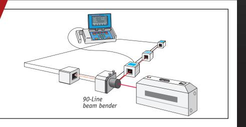
Expand the options for geometric measuring and alignment with the 90-Line Right Angle. The 90-Line redirects the laser beam at a precise right angle, enabling the digital receiver to provide measurements of squareness. Applications include: adjusting the Z axis on machine tools, squaring machinery and equipment, aligning gantry rails and cross bridges, adjusting web and roller systems, checking gantry travel, setting tracks and rails, and positioning machinery.
