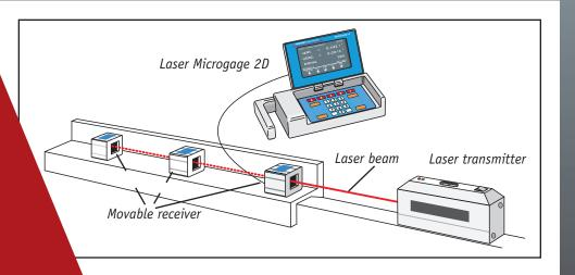
The Microgage 2D receiver detects instantly if a linear run is straight and true. Detect even the slightest deviations in long machinery beds, profile assemblies, measure machinery deflection, track alignment, and more.
