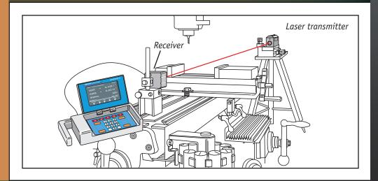
Attach the Microgage receiver to a moving machine slide or assembly and measure the run-out in the travel. Multiple machinery axes can be checked and measurements made over long distant runs. Quickly find worn machinery areas and create compensation tables or use the Laser Microgage to re-align machine travel. High precision readings are ideal for machine tools, printer heads, scanners and other moving mechanical devices.
