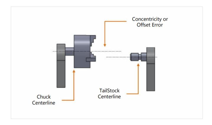
Offset or concentricity misalignments occur when the centerlines of the rotating spindle, chuck, tool holder or work piece holder are displaced from each other. Offset misalignments fall into 2 axes, typically referred to as vertical or horizontal. These centerline or offset errors tend to be fixed and maintain a constant error value as you travel further away from the chuck or tailstock.
