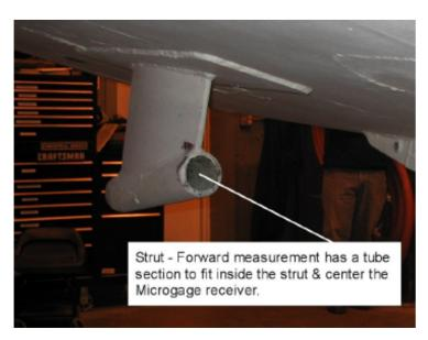
Our recommendation is a tube that is perhaps 3 to 6 inches in length for solid mounting and removal. We have designed plug fixtures for customers and the two photographs above show these fixtures designed for a 1-inch and 2 ¼-inch precision bore. This fixture can be used with the fixture behind the receiver or in front of the receiver in cases where the laser is coming through the center of a bore tube.
