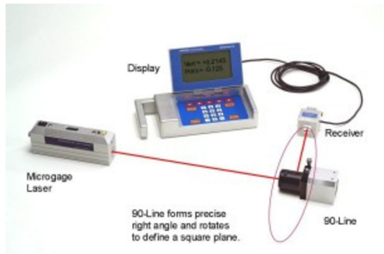
Laser Microgage Checks Roll Parallelism
