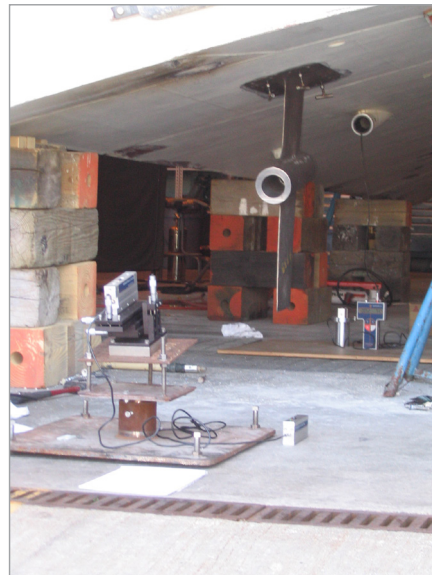
Pitched stand for supporting 4-Axis Mount and laser transmitter
