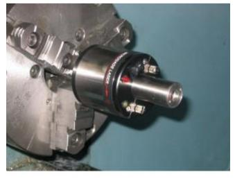
held in the chuck. The laser beam then travels some distance down the length of the machine before it reaches the Microgage Receiver. If the chuck does not grip the laser shank evenly or if there is any reason that the laser doesn't sit squarely in it's mounting
