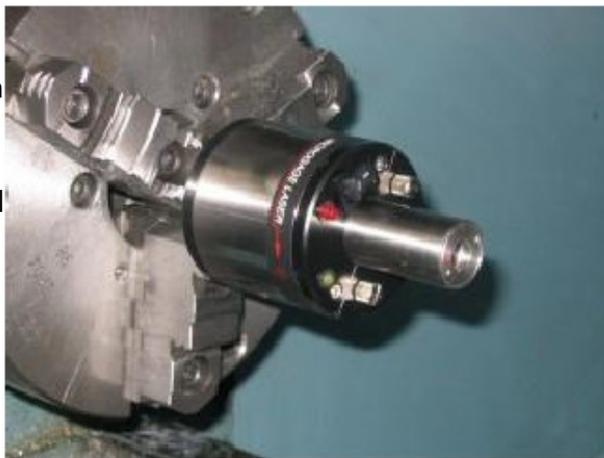
The Microgage Laser typically has a 2 to 3 inch long mounting shank, of a precise cylindrical dimension, that is held in the chuck. The laser beam then travels some distance down the length of the machine before it reaches the Microgage Receiver. If the chuck does not grip the laser shank evenly or if there is any reason that the laser doesn't sit squarely in it's mounting
